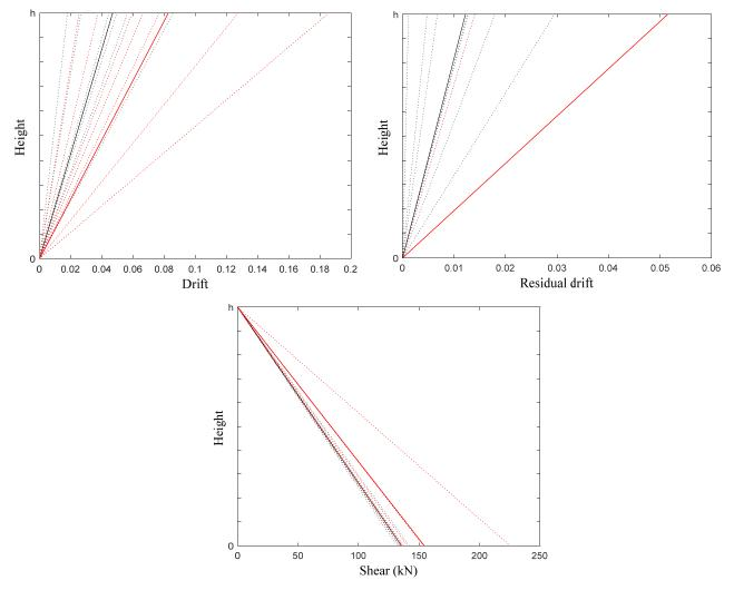
Figure 3. Maximum drift, residual drift and maximum shear of the column subjected to each ground motion (dotty line) and the mean of the responses of the 7 cases (solid line), (Fling step containing: red lines, Far-fault: black lines)
