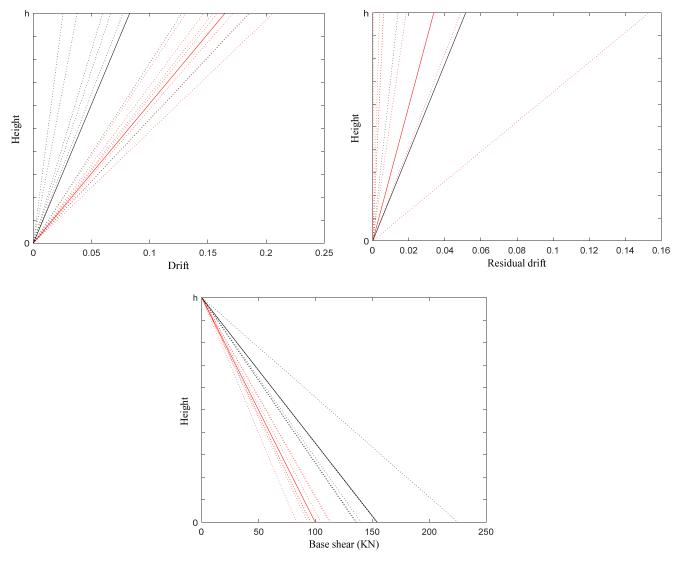
Figure 5. Maximum drift, residual drift and maximum shear of the column subjected to each ground motion (dotty line) and the mean of the responses of the 7 cases (solid line), (SMA: red linnes, No SMA: black lines)
