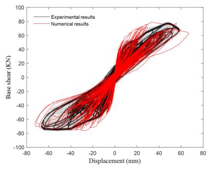
Figure 2. Comparison of the numerical and experimental results.
